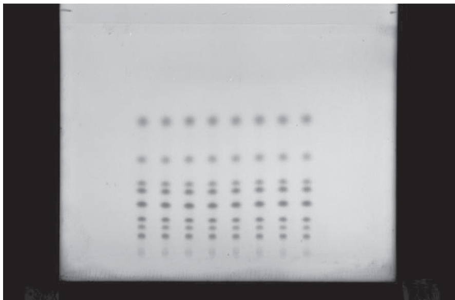
Figure 6 Separation of corticosteroids on silica gel 60 Sorbent layer: HPTLC silica gel 60 F 254 glass plates (Merck) Mobile phase: chloroform/methanol (93 + 7 v/v) Detection: 0.5% w/v blue tetrazolium in methanol Zones: 1, prednisolone; 2, hydrocortisone; 3, prednisone; 4, cortisone; 5, cortico- sterone; 6, cortexolone; 7, 11-dehydrocorticosterone; 8, 11-desoxycorticosterone (from lowest R f ) Concentration: 20 ng per substance
