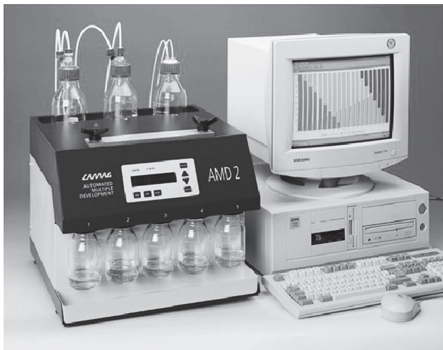
Figure 26 The Automated Developing System (AMD) manufactured by Camag. The developing chamber is situated in the front portion of the unit. The five reservoir bottles under the front housing hold the solvents for use in the developing cycles. Located at the back of the hood is the gas wash bottle, a molecular sieve vessel for making up the gas phase, and a solvent wash bottle. The computer controls any required pre-conditioning, development steps, migration times, solvent concentrations and drying times (Permission for use granted by Camag, Muttensz, Switzerland)
