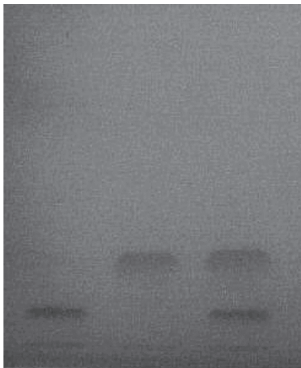
Figure 36 Separation of cis and trans isomers (triolein and trielaidin) of a C18:1 triacylglyceride using argentation HPTLC.
