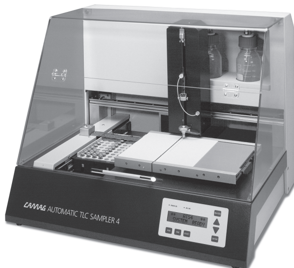
Figure 12 The Camag Automatic TLC Sampler (ATS) 4 for spot and band application of sample solutions from a rack of vials. The operation is programmed and controlled by a personal computer. A standard rack of 66 2 ml vials may be addressed in one application program. Optional special racks hold 96-well plates. The recommended volume range per sample is 100–5000 nl for spots and 2–20 \mu l for bands (Reproduced by permission of Camag, Muttensz, Switzerland)
