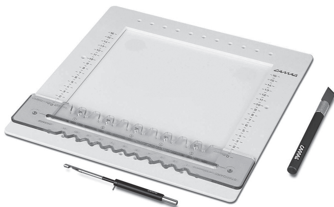
Figure 8 A multi-purpose spotting guide for a 20×20 cm TLC glass plate. One side of the pipette rest has 11 notches, resulting in sample loadings 15 mm apart. Scored lines can be drawn with the tapered pen through the long slit in the pipette rest (Reproduced by permission of Camag, Muttens, Switzerland)
