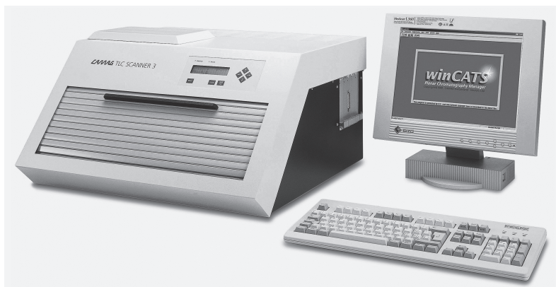
Figure 2 A typical TLC/HPTLC scanning spectrodensitometer. It operates on the basis of a fixed beam of light of selected wavelength and a motor-driven stage holding the TLC/HPTLC layer under the light source. The computer software both controls the scanner parameters and manipulates the vast amount of data produced during a plate scan (Reproduced with the permission of Camag, Muttens, Switzerland)
