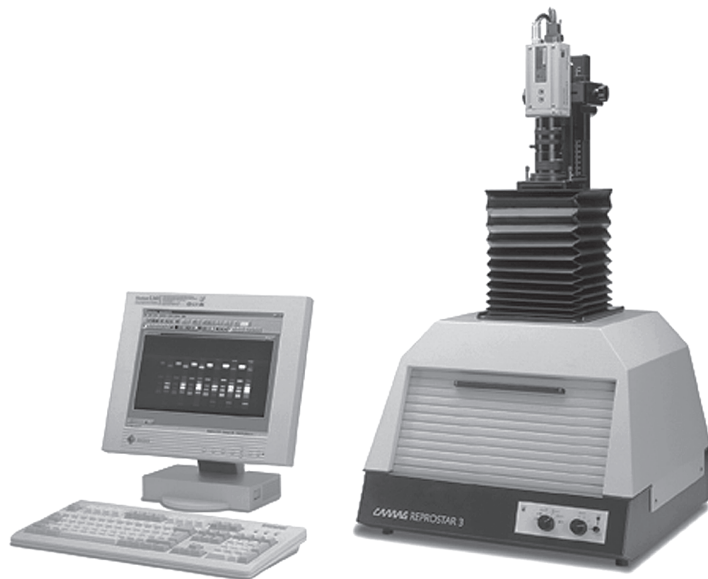
Figure 4 A lighting unit with capabilities of illumination from above and below the TLC/HPTLC layer fitted with a CCD camera and video link to the computer. The computer software controls the camera functions, image enhancement capabilities, and video scanning if required (Reproduced with the permission of Camag, Muttensz, Switzerland)
