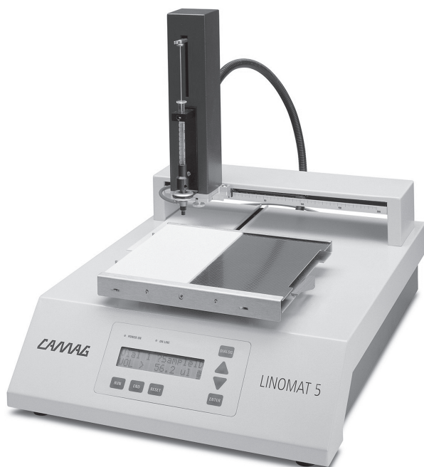
Figure 11 The Camag Linomat 5 for band application of sample solution. This spray-on technique allows larger sample volumes at low concentration to be applied than is possible by contact transfer. Samples are concentrated into narrow bands of selectable length. For preparative purposes, sample solutions can be applied as long narrow bands over most of the plate length (Reproduced by permission of Camag, Muttenz, Switzerland)
