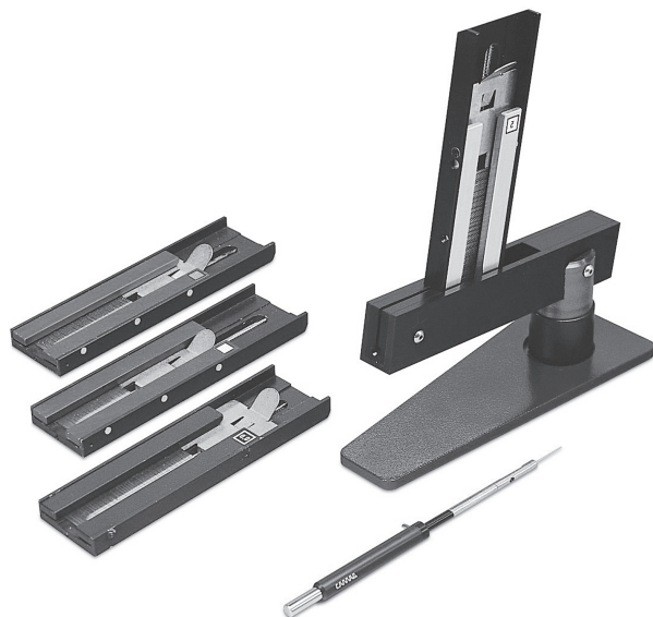
Figure 9 A Camag capillary dispenser unit. The glass capillaries are held in dust-proof dispenser magazines. Capillaries of 0.5, 1, 2, and 5 \mu\text{l} volume are available. To load the capillary holder with a capillary, the magazine is inserted into the dispenser, the holder is pushed into the slotted hole, and then pulled out. The capillary is now in position in the holder. After use, the capillary can be ejected by pressing the end of the holder (Reproduced by permission of Camag, Muttenz, Switzerland)
