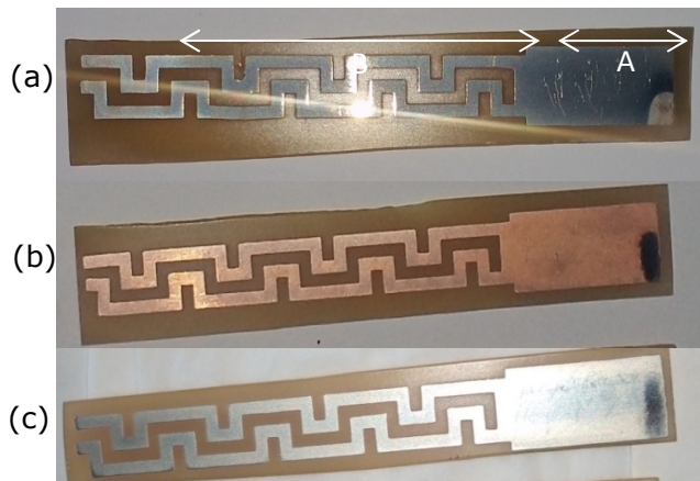
Gambar 15. (a) Lapisan Cu/Ni; (b) Lapisan Cu/Ni/Cu; dan (c) Lapisan Cu/Ni/Cu/Ni. Desain
