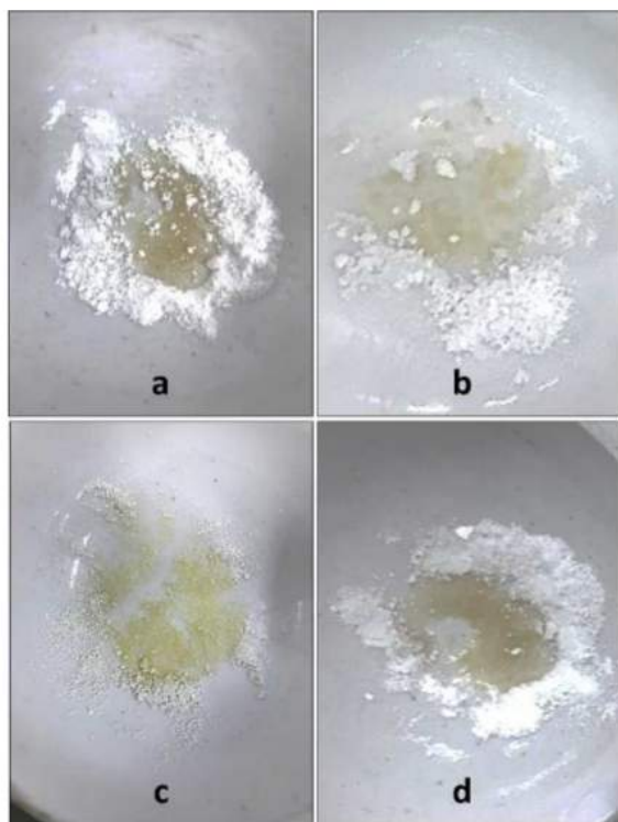
Figure 3. Melted DPC after (a) 20 minutes for MW-assisted-ethanol system, (b) 25 minutes for MW-assisted-methanol system, (c) 40 minutes for MW-assisted-water system, and (d) 45 minutes for neat mixture.
