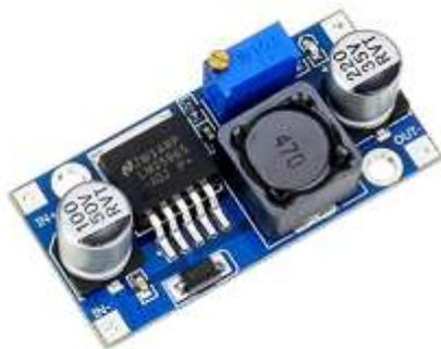
**Gambar 10.** LM2596 DC-DC *Step down*
