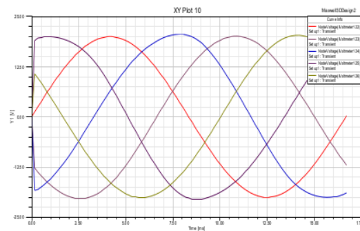
Figure 12. Balanced output of five phase transformer from ANSYS Maxwell
