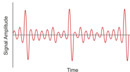
Figure 1. High Peak-to-Average Power Ratio signal in the time Domain [1]
