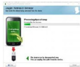
Figure 16. Physical dump Oxygen Forensic process on the suspect's smartphone
