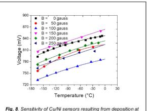
Fig. 8. Sensitivity of Cu/Ni sensors resulting from deposition at magnetic field variations.
