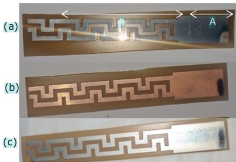
Gambar 15. (a) Lapisan Cu/Ni; (b) Lapisan Cu/Ni/Cu; dan (c) Lapisan Cu/Ni/Cu/Ni. Desain
