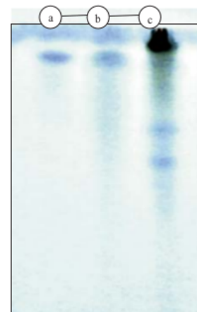
Figure 1. Qualitative identification of the ethanol extract, ethanol extract purified by comparison melatonin. = Silica gel stationary phase and mobile phase = 254 n-butanol: 15% acetic acid: water (12:3:5)
