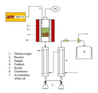
Figure 1. The SPR pyrolysis equipment (Jamilatun et al., 2019)
