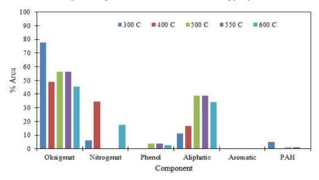
Figure 6. Spectra GC–MS bio-oil from SPR pyrolysis
