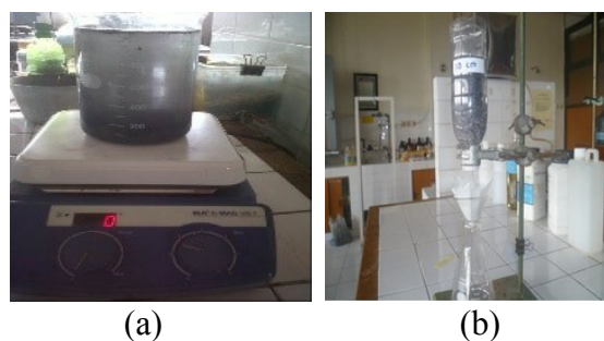
Fig. 2. The purification water by activated charcoal in the laboratory process of UAD: (a) filter column and (b) mixing and stirring
