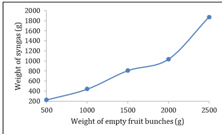
Fig. 3. Relationship between weight of empty fruit bunches and weight of syngas produced
