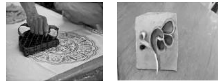
Fig. 1. A. old model Batik cap tool, B. the Batik tool developed
