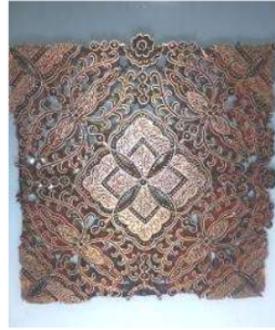
Fig. 2. Metallic flora motif stamp tool. (Source: Studio of the Department of Textile at SMK Negeri 3 Kasihan, Bantul, Yogyakarta Photographer: Probosiwi, 2019)
