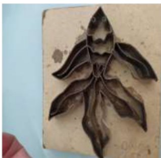
Fig. 15. Fauna batik stamp tool made from duplex paper and hardboard cut. (Source: Studio of the Department of Textile at SMK Negeri 3 Kasihan, Bantul, Yogyakarta Photographer: Probosiwi, 2019)
