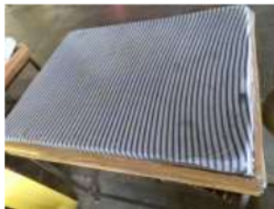
Fig. 8. A wettable that functions as a cloth base that is being stamped with a metal stamp. This table contains cold water that is stacked with a sponge and covered by a blanket cloth and covered by glass paper. The purpose of this table is made so that the process of tasting the fabric is not sticky because it is exposed to cold temperatures from glass paper. (Source: Studio of the Department of Textile at SMK Negeri 3 Kasihan, Bantul, Yogyakarta Photographer: Probosiwi, 2019)
