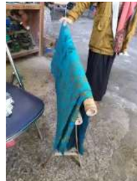
Fig. 11. " Gawangan " is a tool for laying fabric that is being processed batik, can be used as a place to dry batik cloth. (Source: Studio of the Department of Textile at SMK Negeri 3 Kasihan, Bantul, Yogyakarta Photographer: Probosiwi, 2019)
