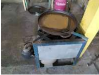
Fig. 6. Frying pan or pan to heat the " Malam " (wax) to taste. " Malam " that has been hot and melted at the top is given a burlap cloth and metal slab that serves as a place to filter dirt. (Source: Studio of the Department of Textile at SMK Negeri 3 Kasihan, Bantul, Yogyakarta Photographer: Probosiwi, 2019)
