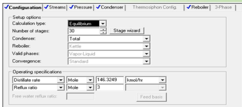
Gambar 4. Configuration of Block RD
