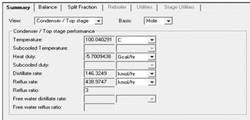
**Gambar 7.** Hasil suhu atas menara Reactive Distillation (Tray Sizing)
