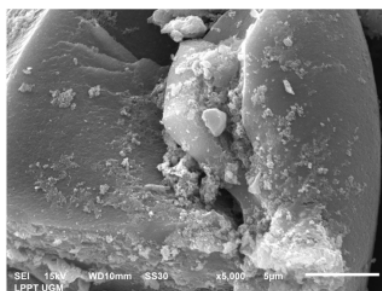
Fig. 1. SEM results for \text{Fe}_2\text{O}_3 /activated carbon catalysts
