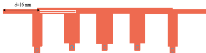
Figure 8. Proposed integrated of bandpass filter with one U-shaped DMS
