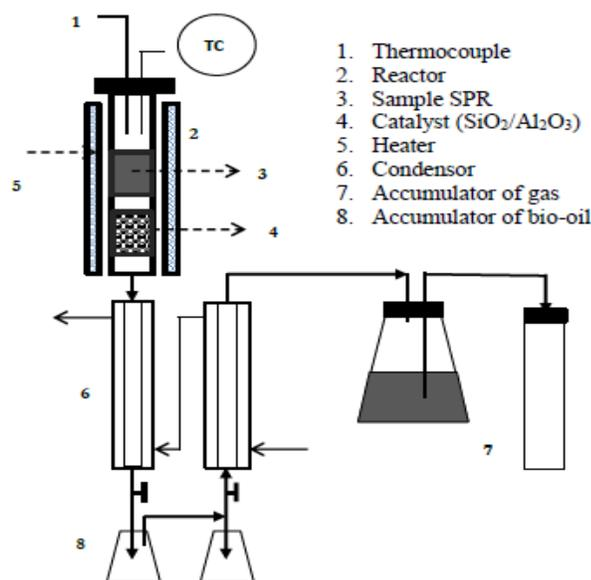
Fig. 1: The schematic diagram of the fixed bed tubular reactor (15)
