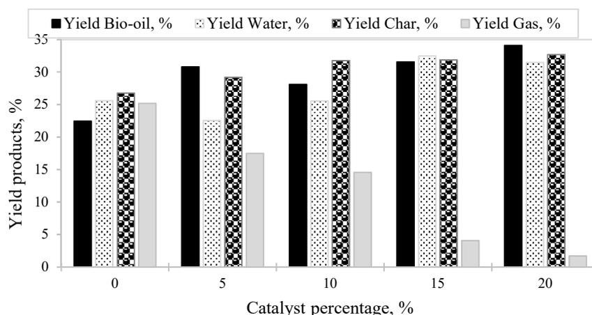
FIGURE 3. The evolution of yield product percentage as function of Si-Al catalyst percentage between 0 and 20% on SPR pyrolysis products at 700 °C
