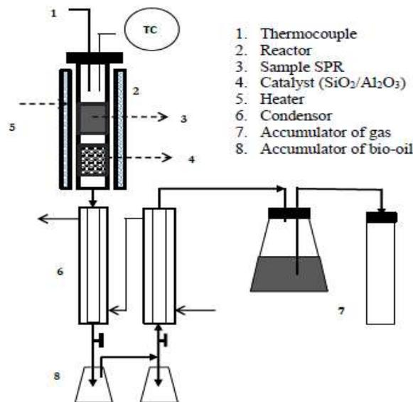
FIGURE 1.: The schematic diagram of the fixed bed tubular reactor
