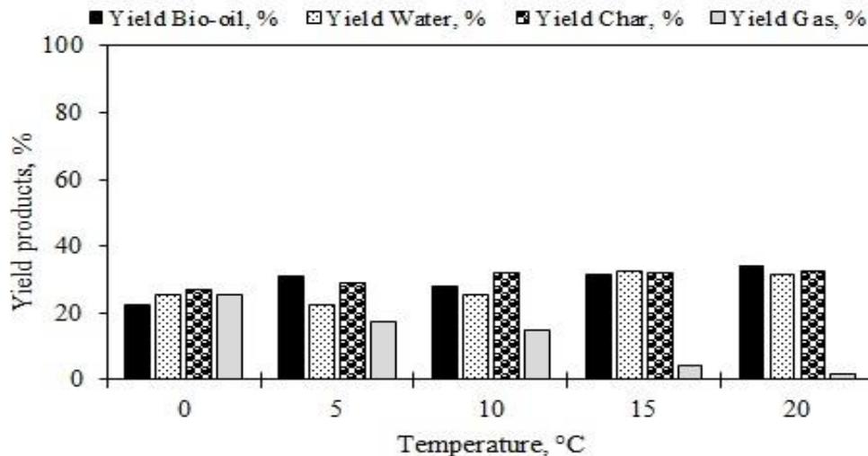
Fig. 3: The evolution of yield product percentage as a function of Si-Al catalyst percentage between 0 and 20 wt.% on SPR pyrolysis products at 700 °C
