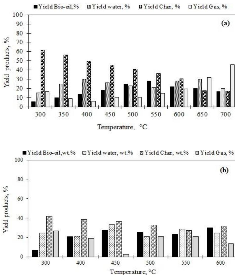
Fig. 2: Effect of temperature on yield products, obtained from SPR pyrolysis process a) without and b) with the presence of 5 wt.% Si-Al catalyst
