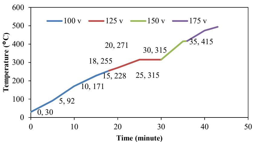
Figure 2. Effect of time on the pyrolysis temperature
