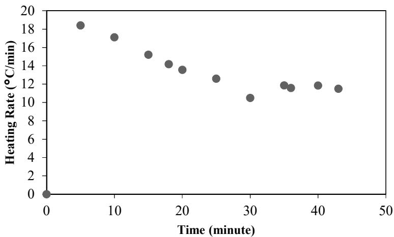
Figure 3. Effect of time on pyrolysis heating rate
