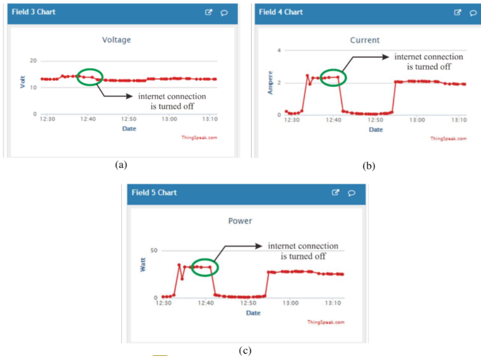
Figure 8. Measurement results (a) voltage, (b) current, and (c) power due to variations in temperature and irradiance
