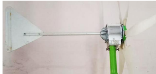
Figure 2. Generator Turbine on PLTH Bayu Baru
