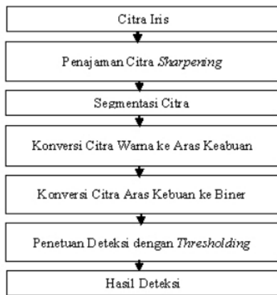
Gambar 2. Diagram blok proses deteksi kolesterol
