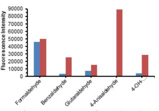
**Fig 7.** Fluorescence intensity of **CHP** ( $1 \times 10^{-4}$  M in acetonitrile) at 480 nm after addition of different aldehyde compounds (200 equiv.) (**blue bars**); the mixture of **CHP** and formaldehyde after addition of other aldehyde compounds (**red bars**)
