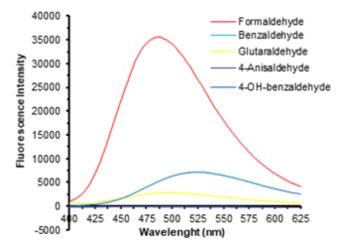
**Fig 6.** Emission spectra of **CHP** ( $1 \times 10^{-3}$  M in acetonitrile) after addition of different aldehyde compounds with excitation at 363 nm
