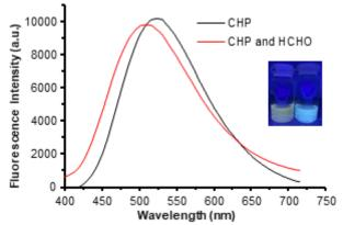
**Fig 2.** Fluorescence spectra of **CHP** ( $2.5 \times 10^{-4}$  M in acetonitrile) before and after addition of 50 µL 37% formaldehyde-water solution with excitation at 363 nm. Inset: Photographs of compound **CHP** ( $2.5 \times 10^{-4}$  M in acetonitrile) before (left) and after (right) addition of formaldehyde under 365 nm portable UV lamp
