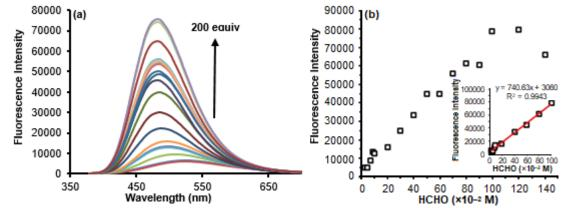
**Fig 3.** (a) Emission spectra of **CHP** ( $2.5 \times 10^{-4}$  M in acetonitrile) upon addition of formaldehyde-water solution (0–200 equiv.) with excitation at 363 nm; (b) Emission intensity of **CHP** at 480 nm as a function of formaldehyde concentration (0–1.4 M). Inset: Linear relationship between fluorescence intensity and the concentration of formaldehyde
