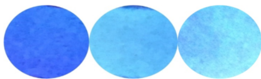
Fig 8. Photographs of probe CHP as test paper for the detection of formaldehyde under 365 nm portable UV lamp (filter paper loaded with CHP in acetonitrile over the water ( left ), formaldehyde ( center ), and application of meatball test ( right ))
