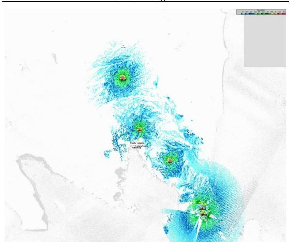
Fig. 8. An example of a display of the simulation results of the prediction coverage area of the radio signal coverage of the repeater equipment for the specific area along 140.938 kilometers
