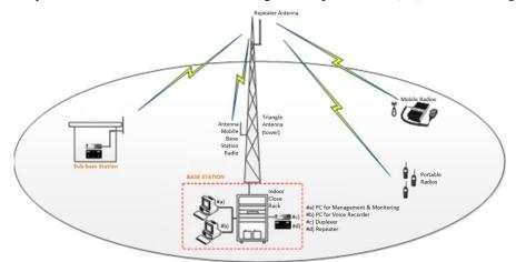
Fig. 3. A schematic diagram of a radio communication system based on DMR Tier-III Trunking for independent use
