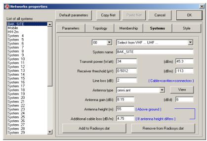
Fig. 7. The display of setting some parameters for determining the predicted radio signal coverage area of the repeater device based on the radio mobile application
