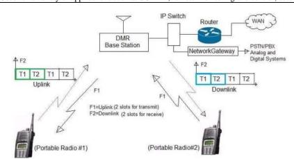
Fig. 2. The schematic diagram of the transmit and receive process on a trunking system
