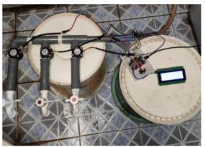
Fig 1. The taps and their water flow sensors
