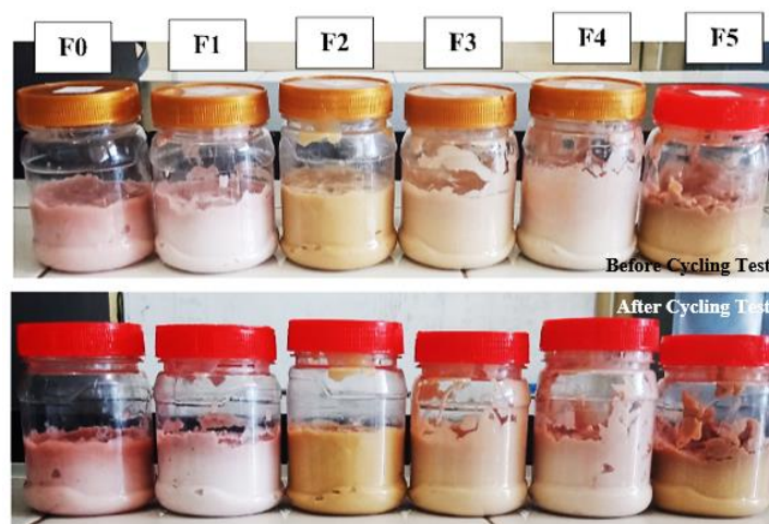
Figure 1. the result of organoleptic test of lotion before and after cycling test. Formula 0 is lotion base; Formula 1 is 100% ZnO; Formula 2 is 100% C. heyneana ; Formula 3 is combination of ZnO- C. heyneana 50:50%; Formula 4 is combination of ZnO- C. heyneana 75:25%; and Formula 5 is combination of ZnO- C. heyneana 25:75%
