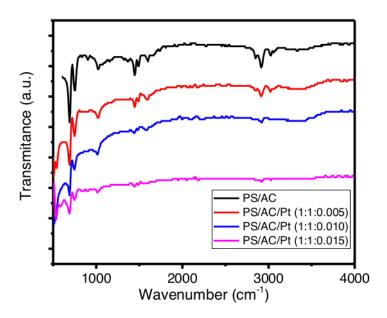
Figure 1. Infrared spectra of the composite materials.
