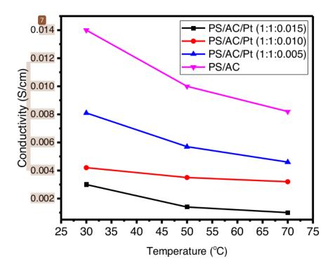
Figure 4. Dependence of the proton conductivity on the temperature.
