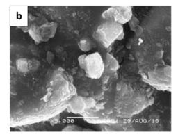
Figure 2. Micrograph of composite material: (a) PS-AC (1:1) g (b) PS-AC-Pt (1:1:0,015).
