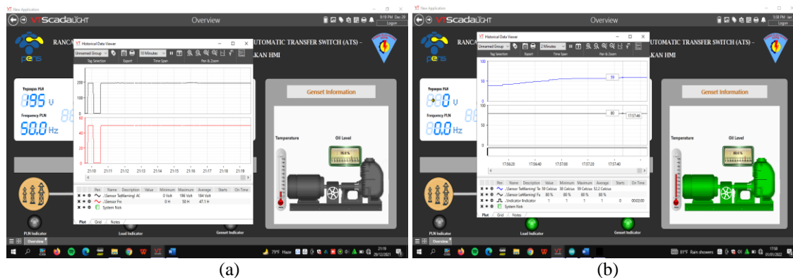
Fig. 8. History Data Viewer, (a) frequency and voltage sensor, (b) Temperature and Fuel Level Sensor
