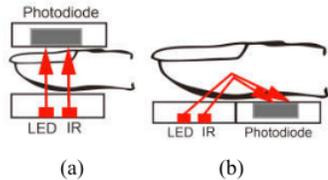
Fig 5. Structure of the pulse rate sensor
