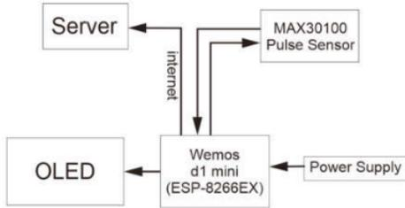
Fig 4. Block diagram device
