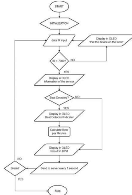
Fig 7. Flowchart Sensing Process
