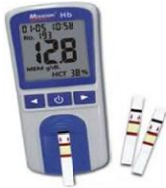
Gb 4. Hemoglobinometer/ Hb meter
