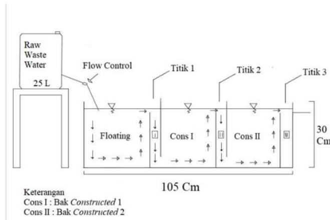
**Gambar 1.** Skema reaktor *floating* dan *constructed wetland*.
