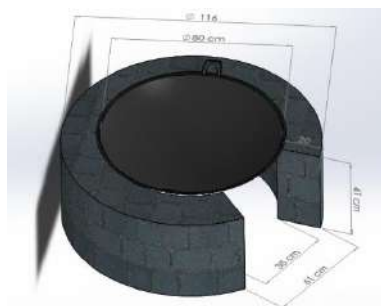
Figure 8. Dimensions of the Cooking Stove and Cauldron of Dodol
