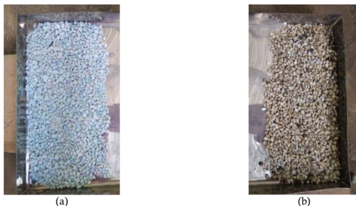
Figure 6. The zeolite catalyst in the system (a) before running (b) after running
