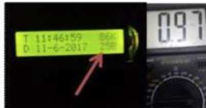
Figure 6. Display of moisture sensor on 16x2cm screen of LCD and multimeter
