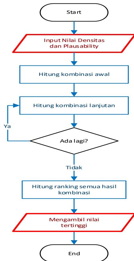
**Gambar 2.** Flowchart perhitungan *dempster shafer*
