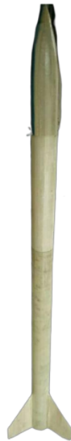
Figure 2. Design of a water rocket from carbon fiber with a tube diameter of 20 mm and the body length of the water rocket is 170 cm
