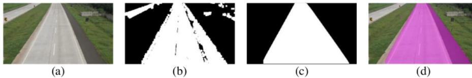
Fig. 4. The result of road area extraction (a) Road frame (b) Road pixel extraction result (c) Road shape estimation result (d) Road area extraction on frame (magenta color marker).
