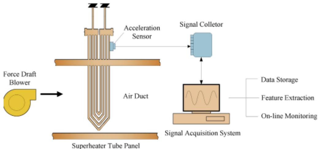
Fig. 5. Experimental setting of Slagging Diagnosis based on tube panel vibration signal
