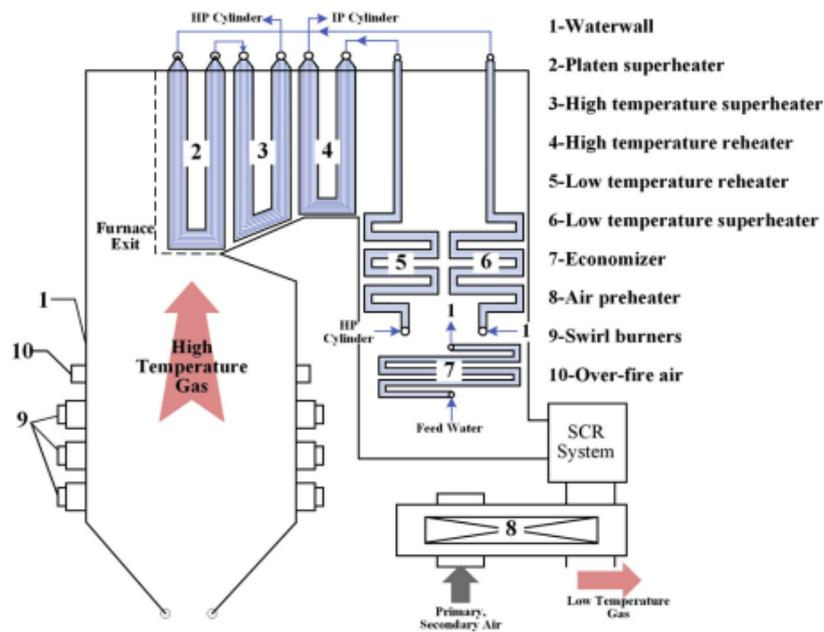
Fig. 1. Boiler Usage Flowchart
