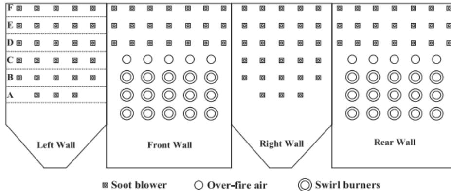
Fig. 3. Burner arrangement
