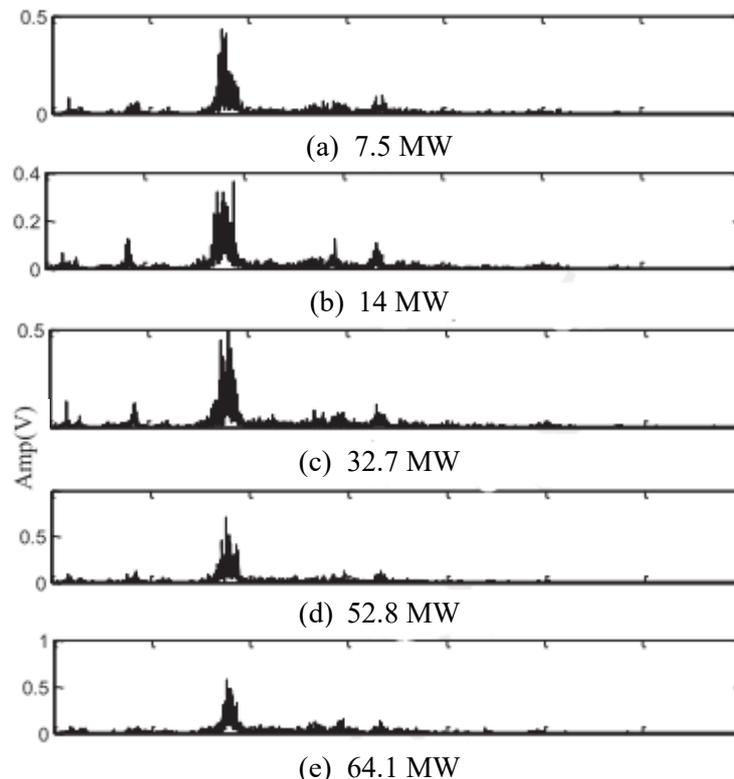
**Fig. 9.** Heating panel signal amplitude spectrum with variable boiler load
