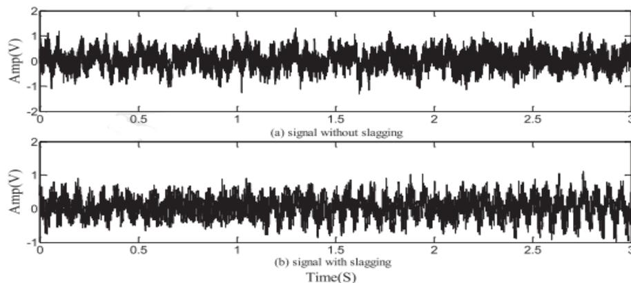
Fig. 6. The time domain waveform of the tube panel vibration signal in the laboratory
