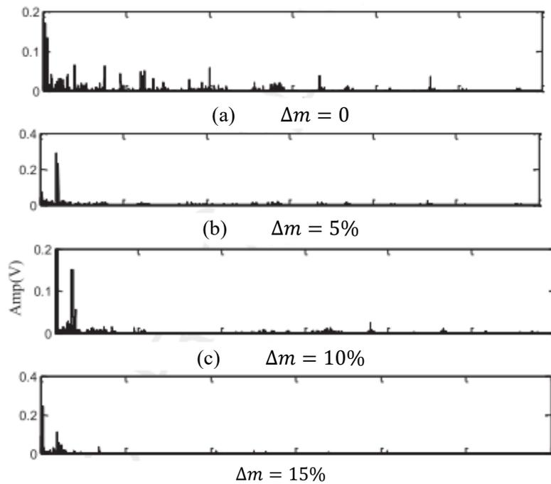
**Fig. 8.** The amplitude spectrum of the tube panel signal under different slagging conditions at an air speed of 12 m/s.
