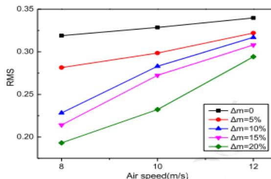
Fig. 7. RMS value of tube panel signal with variable slagging weight and air velocity
