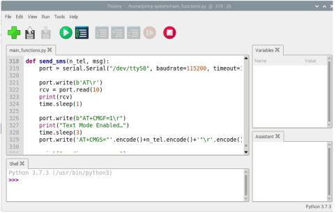
Fig. 11. Samples of some used AT commands
