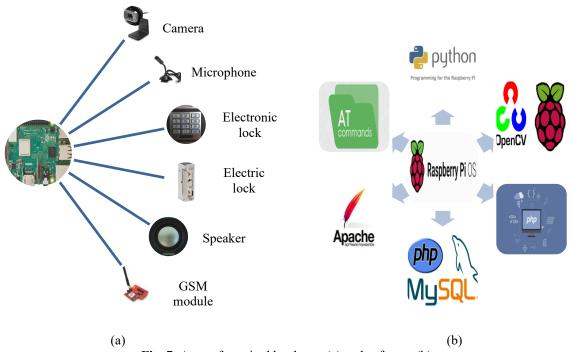
**Fig. 7.** A set of required hardware (a) and software (b)
