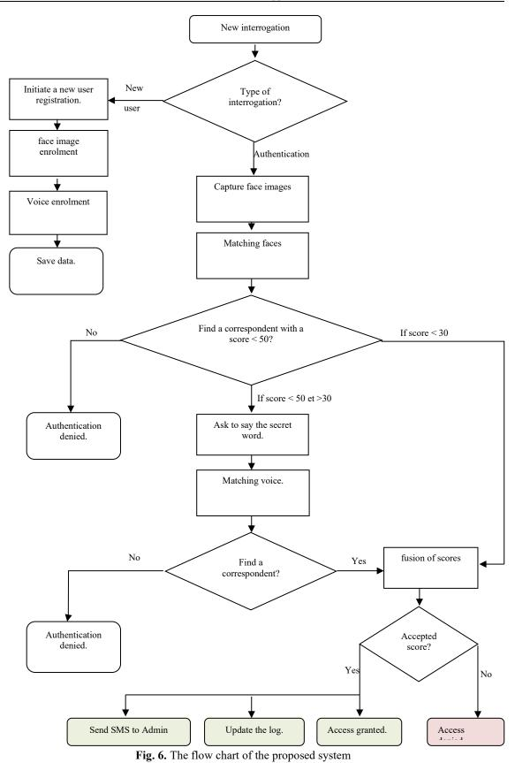
Design and Implementation of Embedded Biometric-Based Access Control System with Electronic Lock using Raspberry Pi (Youssef Elmir)
