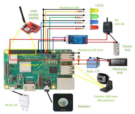
Fig. 10. Components connection schema
