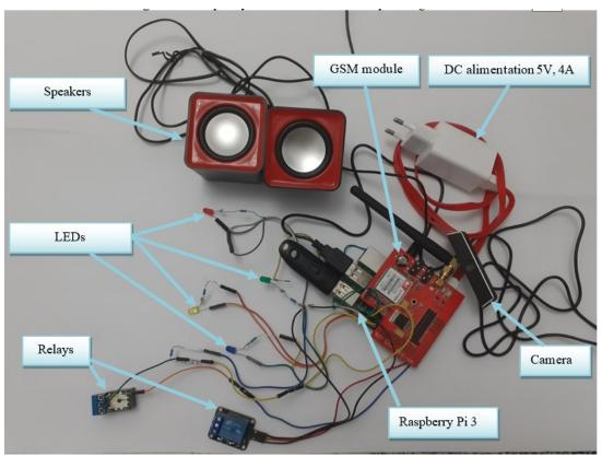
Fig. 9. The connection of the different components of the proposed system
