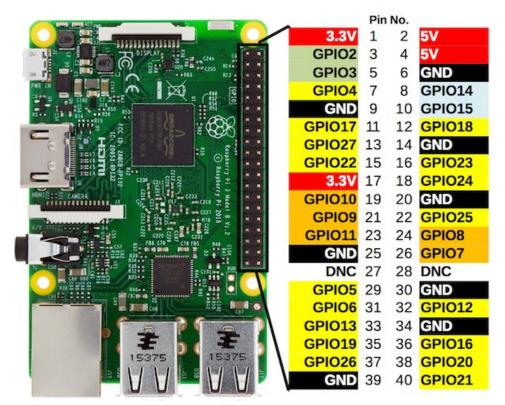
Fig. 8. The Raspberry Pi 3 board with a GPIO port diagram
