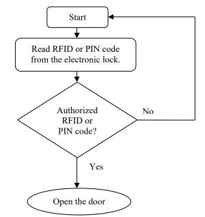
Fig. 3. The operating mode of the existing system at SGRE-Lab
