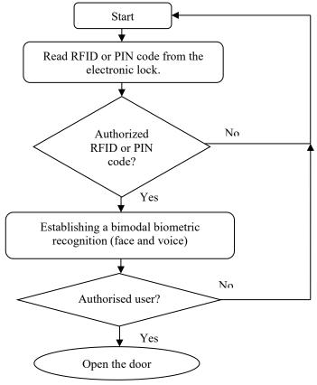
Fig. 5. The operation mode of the proposed system
