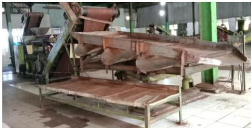
Gambar 1.14. *Rotary Roll Breaker* (RRB) III
