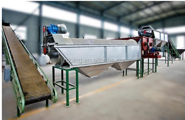
Gambar 1. 22. Mesin Cuci Ubi Tipe Rotary.
