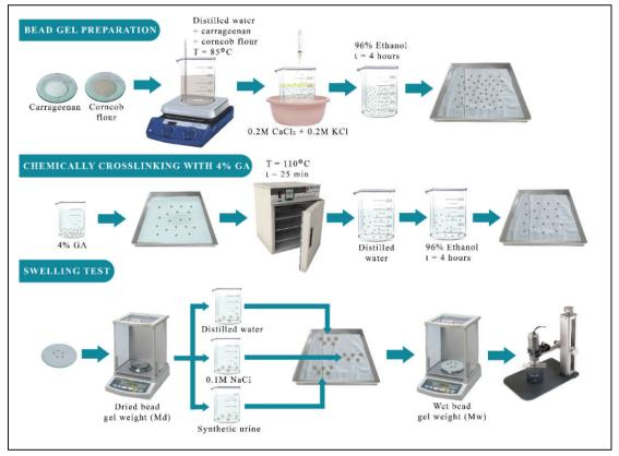
Fig. 2.Process of bead gel preparation, chemically crosslinking, and swelling test
