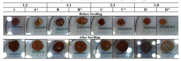
Table 4. The vision under the digital microscope (dino-lite) of the bead gels morphology in synthetic urine
