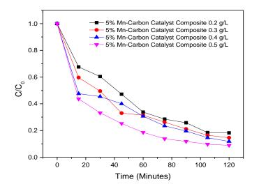
**Fig.3.** Degredation performance of the Mn/Carbon sphere catalyst at different catalyst mass MB = 25 mg/L, PMS loading = 1.0 g/L, and T = 25 °C.
