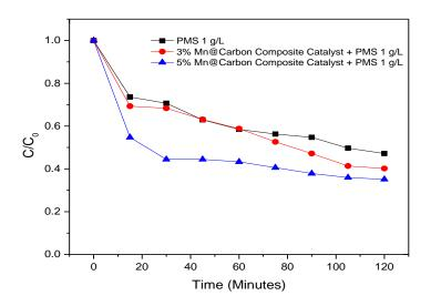
**Fig.2.** Degradation performance of the Mn/Carbon sphere catalyst at different Mn content. MB = 25 mg/L, catalyst loading = 0.1 g/L, PMS loading = 1.0 g/L, and T = 25 °C.
