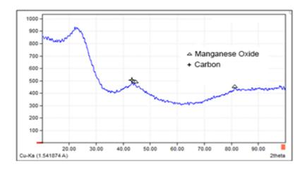
Fig.1. XRD pattern of the catalyst Mn/Carbon sphere Composite.
