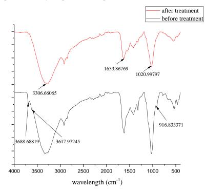
Fig. 3. Results of FTIR analysis of Apu wood root adsorbents (native) before and after treatment
