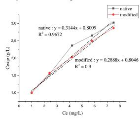
Fig. 6. Langmuir adsorption isotherm of Apu wood root and modification of Apu wood roots
