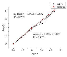
Fig. 7. Freundlich adsorption isotherm of Apu wood root and modification of Apu wood root
