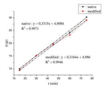
Fig. 9. Reaction kinetics of Pseudo 2<sup>nd</sup> Order adsorption of Apu wood root and modified Apu wood root
