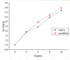
Fig. 1. Effect of initial concentration on the adsorption capacity of Apu wood roots and modification of Apu wood roots
