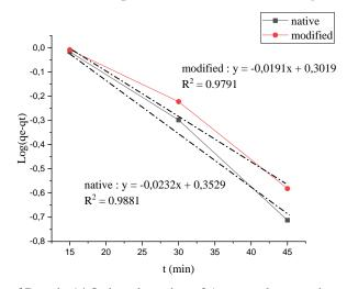
Fig. 8. Reaction kinetics of Pseudo 1<sup>st</sup> Order adsorption of Apu wood root and modification of Apu wood root
