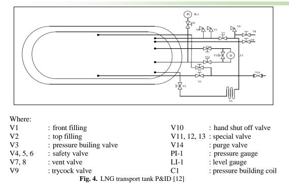
Based on Figure 4, other scenarios that cause LNG release can also be made because the level indicator fails to work, the pressure indicator fails to work, the pressure regulator fails to work, the vent valve fails to open, the filling valve fails to close, the safety valve fails to open, and the operator fails to see pressure/level indicator failed to take action.
