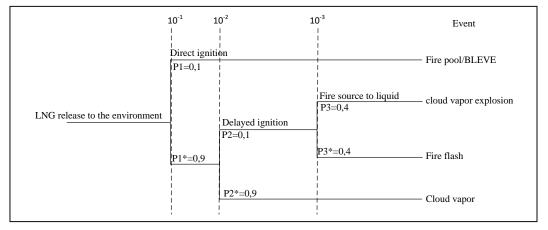
**Fig. 6.** ETA of releases LNG to the environment[15]
