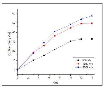
Fig. 3. Cobalt recovery during bioleaching experiment
