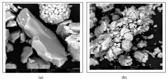
**Fig. 4.**LiCoO<sub>2</sub> Surface Morphology: (a) before bioleaching, (b) after bioleaching
