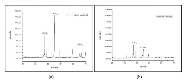
**Fig. 5.**XRD analysis of original LiBs powder of particle size <100 mm. (a) before bioleaching; (b) after bioleaching
