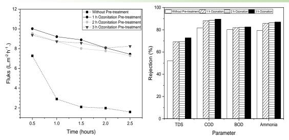
Fig. 5. PES-nano ZnO membrane performance: a). Flux b). Rejection
