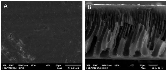
Fig. 3. SEM results of the PES-nano ZnO membrane
