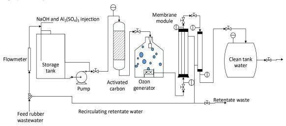
Fig. 1. Applied technology flow diagrams for rubber wastewater treatment
