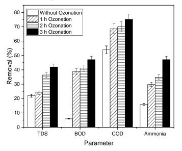
Fig. 4. Impact of ozonation time on waste parameters
