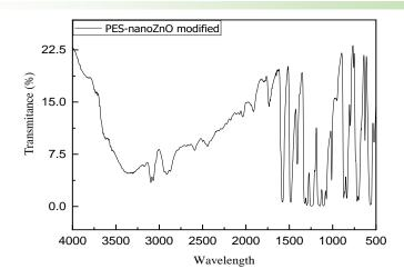
Fig. 2. The FT-IR spectrum of PES-nano ZnO membrane
