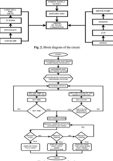
Fig. 3. Sensor reading flowchart
